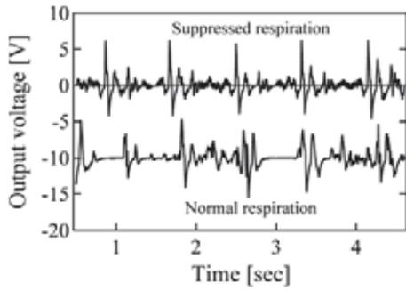
(b) Cardiorespiratory detection results using the **bending-insensitive** mode PVDF sensor, which is attached to the chest, when the person is with normal respiration and with suppressed respiration, respectively
