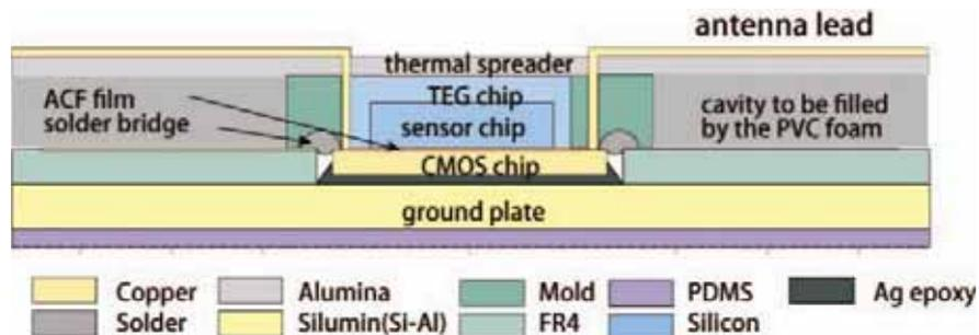
(b) Side view (cut) of the central 10mm section of the proposed Bansoko device
