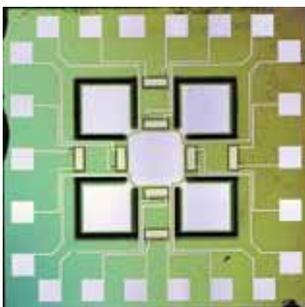
(a) Hybrid accelerometer (removed counter electrode)
