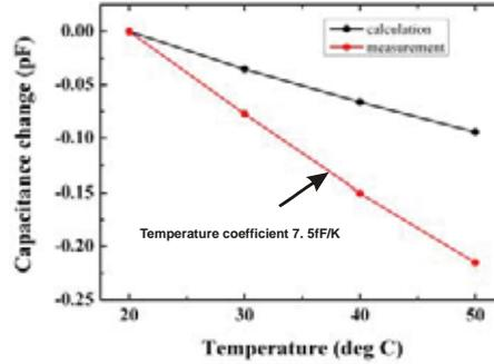
(b) Capacitance VS. Pressure      Capacitance VS. Temperature
