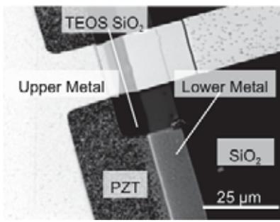
(b) wiring over PZT step (Upper Metal)
