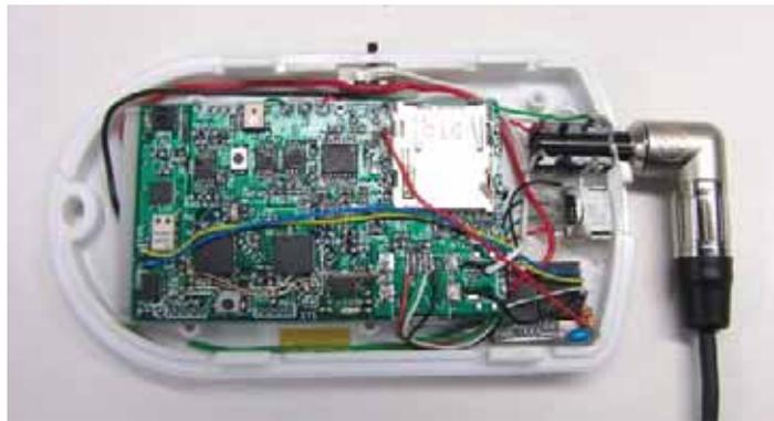
(a) LM03 (SD Memory, USB interface, Bluetooth interface and sensors with 3D acceleration, Humidity, Pressure, Temperature, ECG and Sound)
