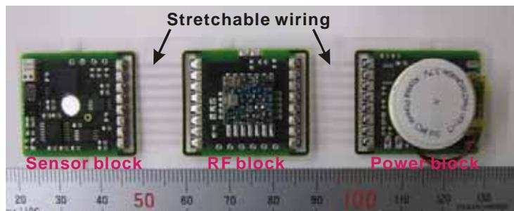
PCB (Left): 3-axis accelerometer, pressure, humidity, temperature sensor, ECG amp and microcontroller
