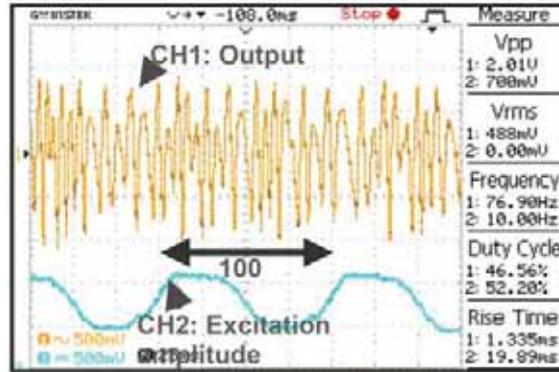
Voltage waveform during power generation.
