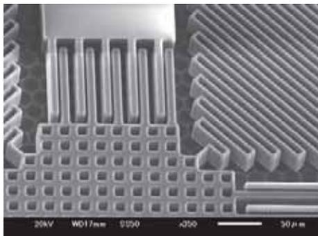
(a) 3-D comb structured accelerometer
