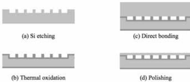
Si on Honeycomb SiO2 process flow
