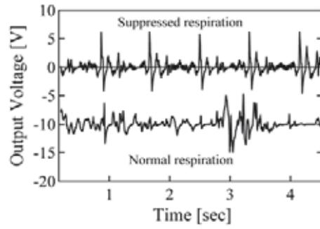
(c) Cardiorespiratory detection results using the **bending-sensitive** mode PVDF sensor shown in the above figure, when the person is with normal respiration and with suppressed respiration, respectively.
