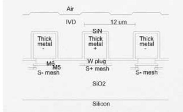
The top metal layer of a CMOS LSI is used as a humidity sensor
