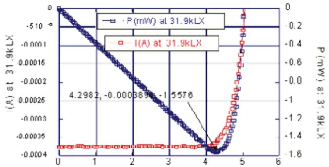
(b) Ten solar cells in series exposed at 31.9 kLX light (This condition roughly corresponds to the shade area in a fine day)
