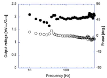
(c) Frequency response of PZT accelerometer
