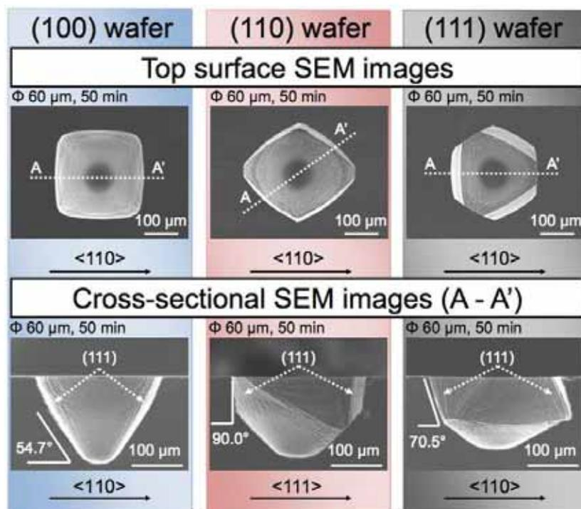
**(5) TSV and wiring by anisotropic Si dry etching**
