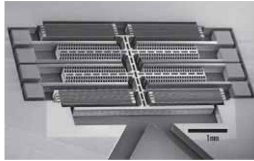
(b) Comb structured electrostatic actuator
