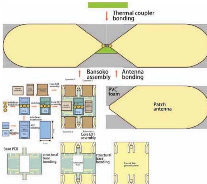
(a) Top view of the main components and the Bansoko assembly
