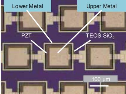
(a) Cascade connected PZT device
