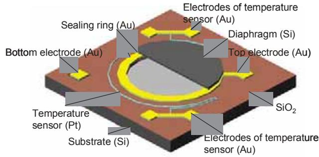
(a) Schematic structure of the pressure sensor
