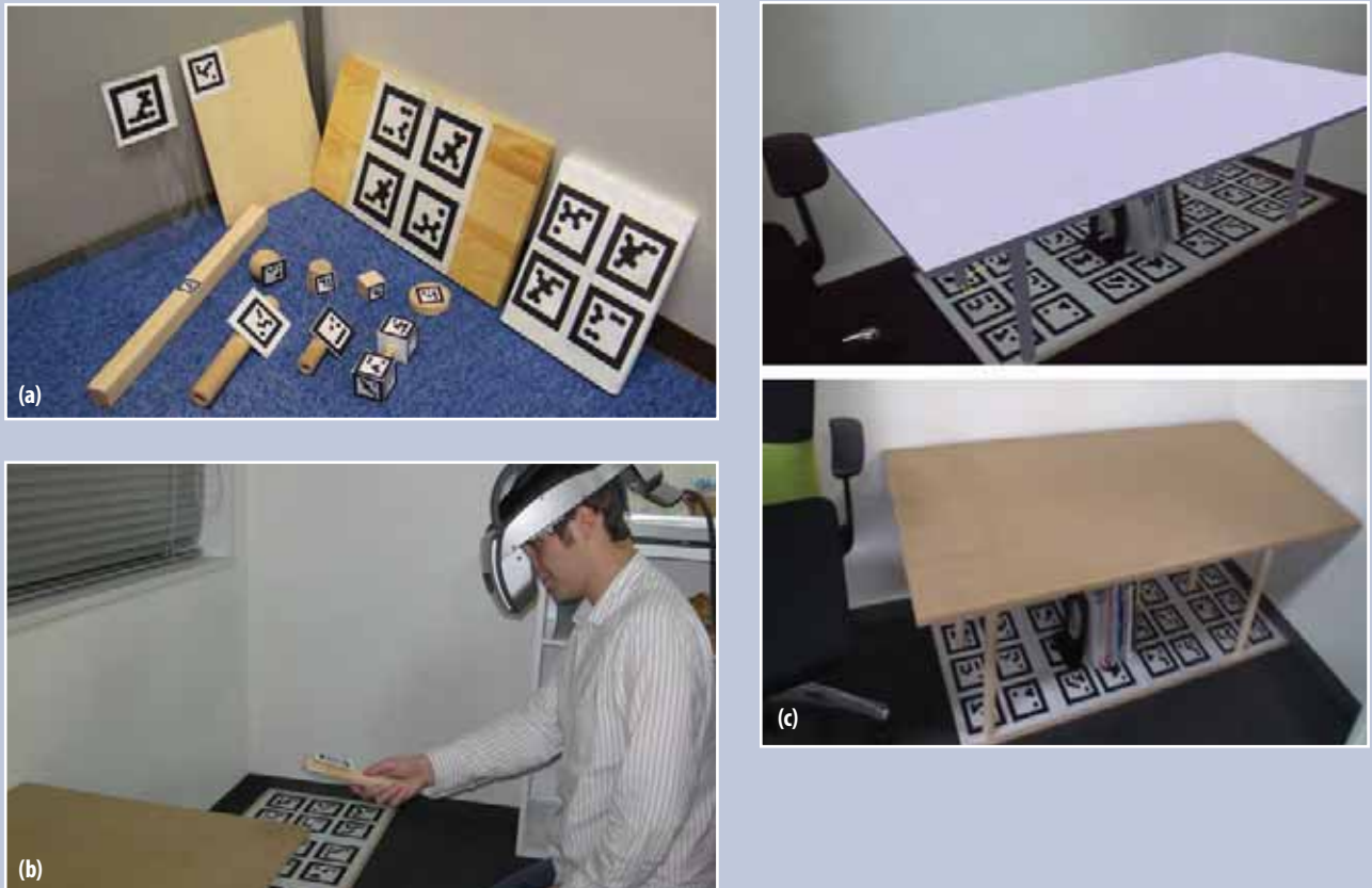
Figure 2. Using situated modeling to design a table to fit in the empty corner of a living room: (a) tangible primitive wooden shapes with markers for identification purposes; (b) a user wearing the head-mounted display and holding one of the shapes; (c) digital table model created by the system, and corresponding physical table later assembled from wood pieces.
