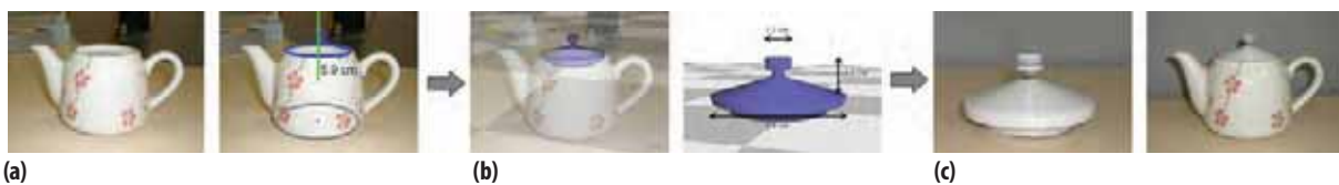
Figure 1. Using modeling-in-context to design a replacement lid for a teapot: (a) original photo of the teapot and 2D user sketch and annotations of the new lid; (b) 3D digital model of the new lid; (c) new physical lid from 3D printer that fits well with the original teapot.
