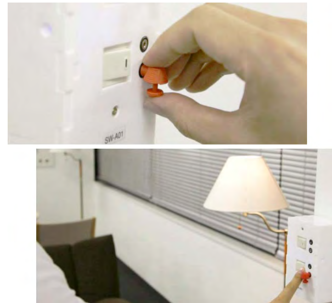
figure 1. Tangible pin associated with floor lamp inserted into a pin slot of switch, to control the floor lamp.
