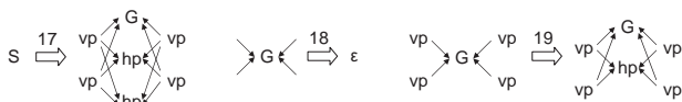
Figure 3: Extra production rules for 3D cabinets. Note that these extra rules are in the same grammar as the one in Figure 2. vp represents a vertical-panel part, h represents a horizontal-panel part, and G is for adding more horizontal-panel parts.
