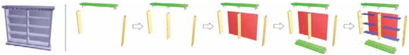
Figure 6: Model m844 (left) from the Princeton Shape Benchmark, and assembly instructions generated from our grammar. The focus of our work is to generate fabricatable parts and connectors, but our approach can also generate assembly instructions.
