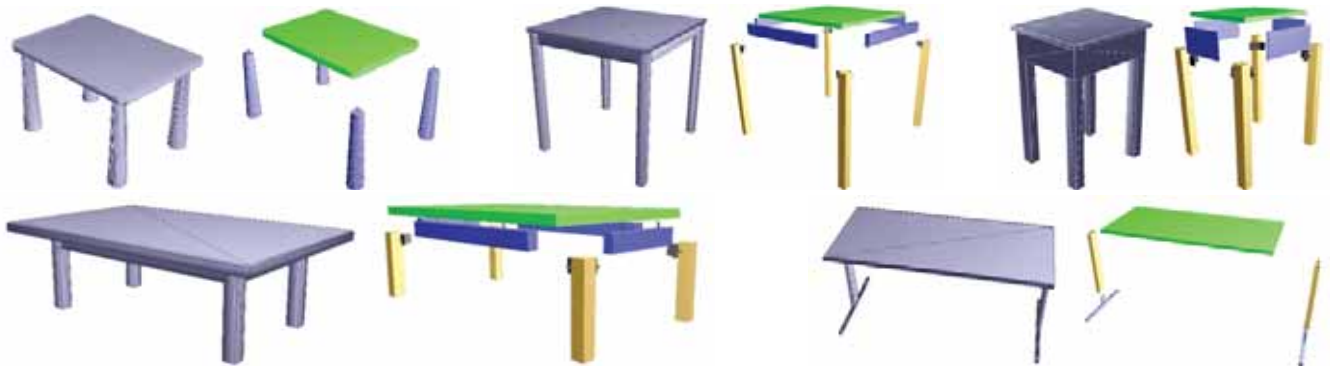
Figure 8: Input 3D models and fabricatable parts/connectors generated by our algorithm for two IKEA table models (MAMMUT, NORDEN) from Google 3D Warehouse and three arbitrary table models (m871, m895, m907) from the Princeton Shape Benchmark.
