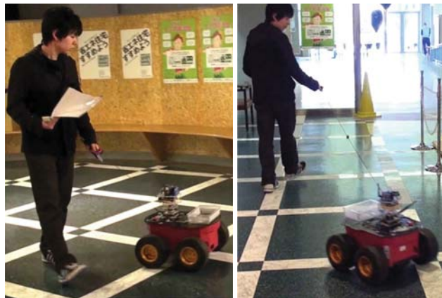
Figure 1 – leading the dog-leash robot: robot in front (left) and robot behind (right)
