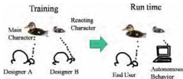
Figure 1: First the behavior of a reactor is demonstrated in response to a main character's behavior. At run time, the reacting character's behavior is synthesized, reproducing the personality and emotion demonstrated in the training.
