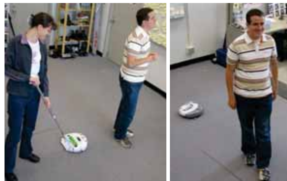
Figure 1. Style by demonstration: (left) a person uses a broomstick interface to show the robot a specific style of interactive movement (in this example, follow politely ), and (right) the robot mimics the demonstration to follow politely.
