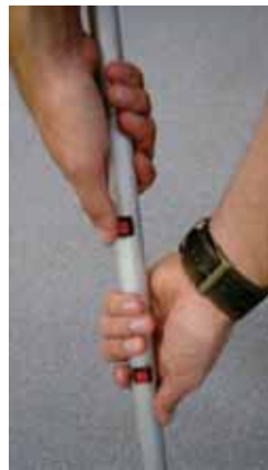
Figure 9. Broomstick-Roomba interface, with mounted buttons.
