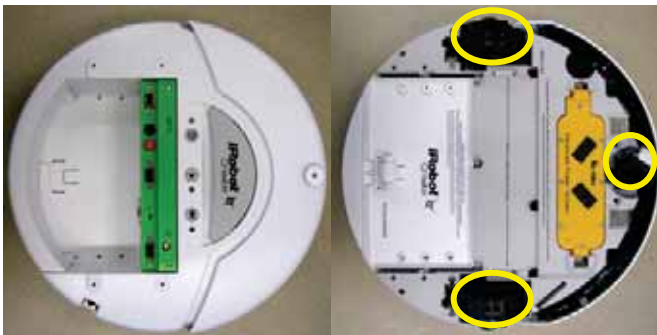
Figure 2. iRobot Roomba, with underside view: two-wheel base and coaster highlighted.
