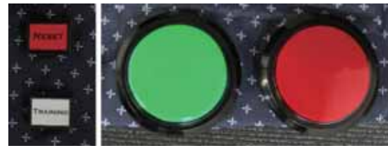
Figure 3. various buttons on the Puppet Dancer interface: the “reset” button erases demonstration data, the “training” button toggles between authoring and playing modes, and the large green and red buttons are the approve and disapprove reinforcement buttons, respectively.
