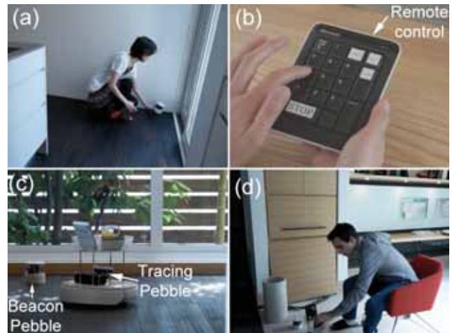
Figure 1: Pebbles: (a) The user places the pebbles on the floor. Each pebble has a unique ID and can communicate with the adjacent pebbles. (b) The user sends the robot to a destination by pressing a labeled button. (c) The robot is navigated by beacon pebbles. (d) The robot arrives at the goal.
