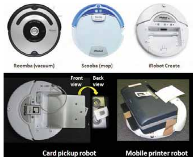
Fig. 6: At top are photos of various robots from iRobot used in project. At bottom are card pickup robot and mobile printer robot modified using iRobot Create.
