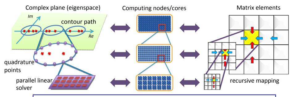
Cluster computing nodes and cores according to hierarchical structures of the
