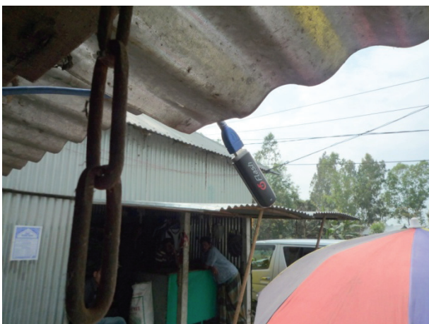
A GSM modem connected to a PC's USB port. The modem is raised as high as possible because the radio waves are weak. The modem is hung from the roof.
