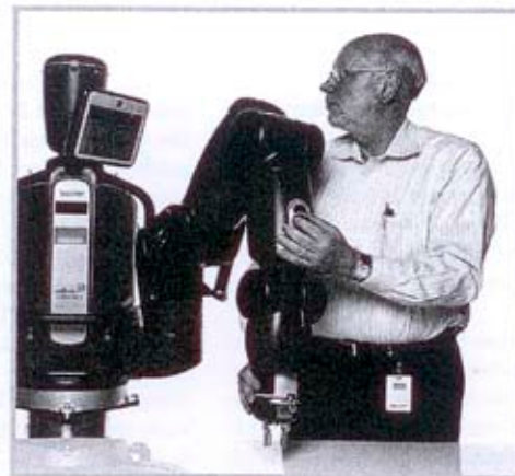
PROGRAM ME, PLEASE: Product manager Mike Bugda demonstrates how to program Baxter to perform a new task. He simply holds the arm by the cuff and moves it to the desired location. He tells the robot what to do using a knob and buttons.
