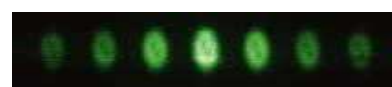
(Fig. 1) The picture of diffraction pattern. Brightest spot is the 0 th order peak.
