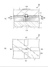
electrode 5A and the other electrode 5B that are provided to have a nanogap, a metal nanoparticle 7 arranged between the electrode 5A and the other electrode 5B in insulated state, and a plurality of gate electrodes 5C, 5D, 11, 11A, 11B for adjusting a charge of the metal nanoparticle 7. Electric current that flows between the electrode 5A and the other electrode 5B is controlled in accordance with the voltage applied to three or more of the gate electrodes 5C, 5D, 11, 11A, 11B.
