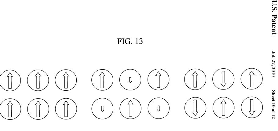
(a) FERROMAGNETISM (b) FERRIMAGNETISM (c) ANTIFERROMAGNETISM
