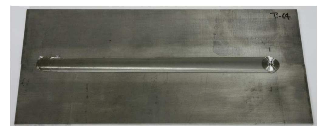
Fig.4 Welded Sample (Two Ti plates are welded)
