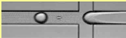
Fig.2 Micro droplets formation in the + intersection
