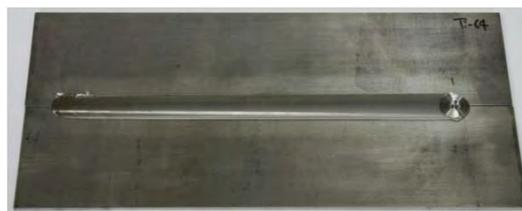
Welded Sample (Two Ti plates are welded)
