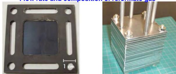
MPOX reformer module comprising of CSO.15MFO and ZMG232R (left) and its 20 stacks (right)
