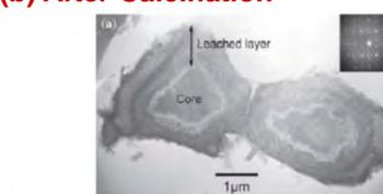
a) BFI of cross-section of NaOH leached Al-Cu-Fe QC alloy after calcination at 600°C
