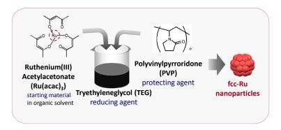
Particle size is controllable by varying the synthesis condition.
