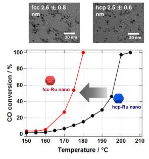
Condition: Catalyst Quantity :  $0.075 \, \mathrm{g}$ ,  $\mathrm{Al_2O_3(\gamma)}$ -supported Ru Reaction Gas :  $\mathrm{He/CO/O_2} = 49/0.5/0.5$  (cc/min) Reaction temperature :  $150 \, ^{\circ}\mathrm{C} \sim$
