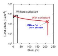
(b)Conductivity vs Strain
