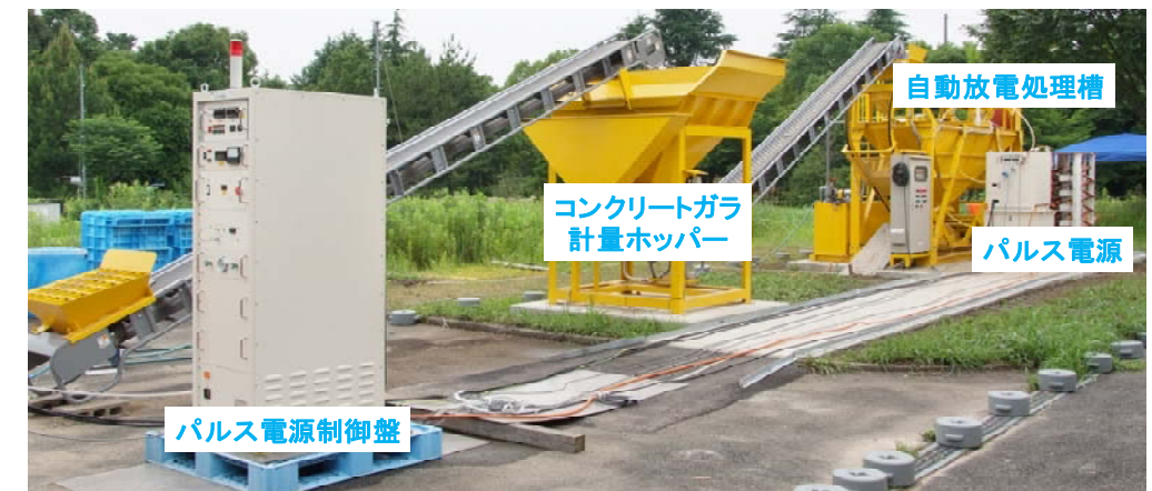
図3 PULSAR-Mk.I (PULSed power based Aggregate Recycler)
