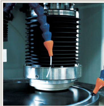
Polishing agent is dripped onto the surface
