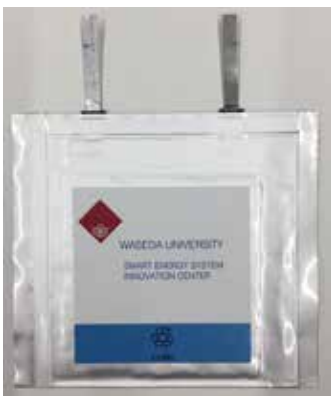
Realizing discharge capacity of 1 Ah/cell using an electrode carrying sulfur of 17.5 mg/cm 2 .
