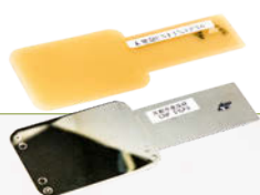
Electroless plating can also be applied to the polymer foams.
