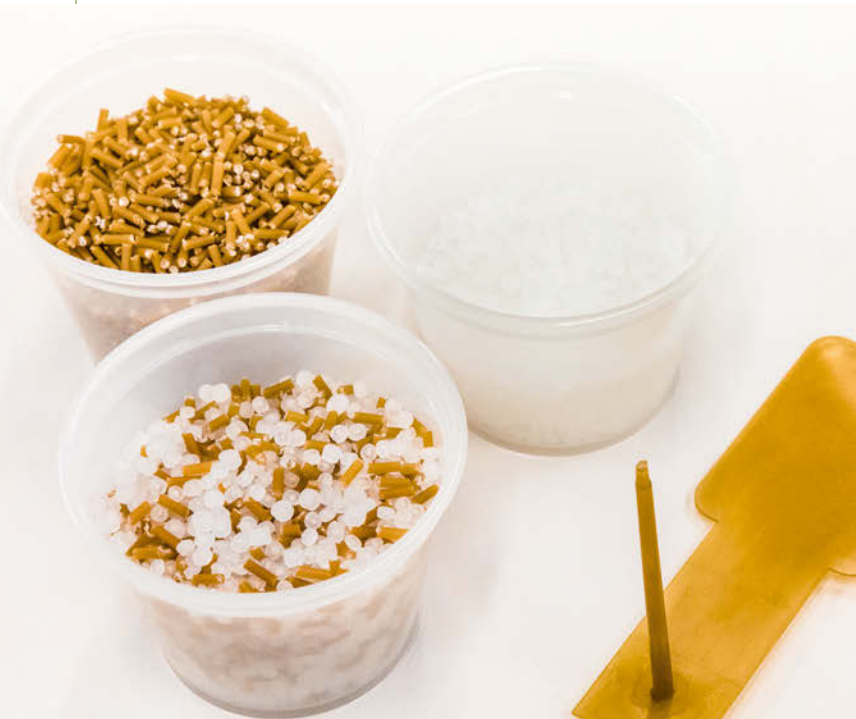
The mixture of CNF-PP masterbatch (brown) and virgin polypropylene (white) pellets is fed into the foam injection molding machine and foamed.
