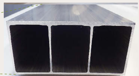
Large size hollow material prototype of mock car bumper reinforcement component
