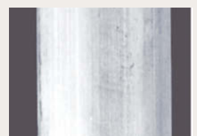
Extruded material: extruded at a temperature of 500°C. High-speed extrusion at the outlet velocity of 60 m/min is possible.
