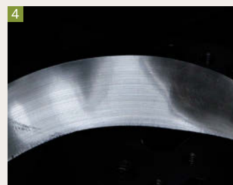
1 Lithium vacuum casting apparatus 2 Lithium extruder 3 Lithium rolling mill 4 Extruded lithium metal foils
