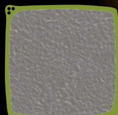
Realizing lithium films with less pits (abnormal grain growth during electrodeposition process)
