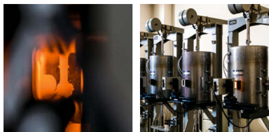
A creep test, applying a constant tension load to the materials at a high temperature.
