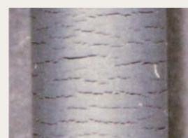
Extruded material: extruded at a temperature of 500°C. High-speed extrusion at the outlet velocity of 60 m/min is possible.
