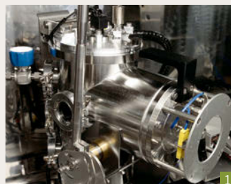
Ultra-high vacuum lithium vapor deposit system for controlling the crystalline orientation of lithium foils.
