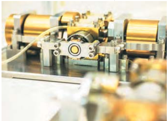
Vibrationless cross balance reciprocal expander unit used for a trilateral steam cycle
