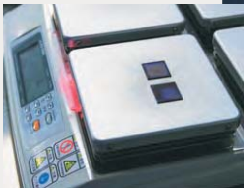
Thermal annealing of a perovskite film on a hotplate
