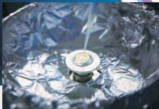
Perovskite film casting by spin-coating method
