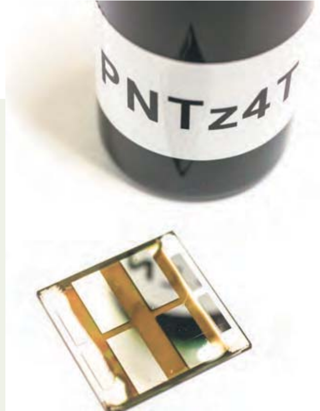
Developed polymer ink (above), solar battery manufactured by painting (below)
