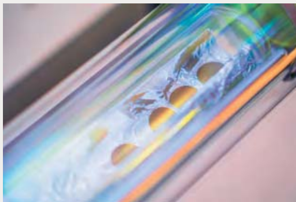
A cathode for trial-manufactured batteries during the drying process
