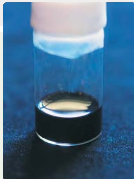
Cathode pseudocapacitive material with high capacitance (colloidal solution of ruthenium oxide nanosheets)
