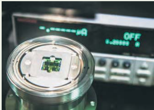
Measurement of the properties of a solar battery by irradiation with simulated sunlight
