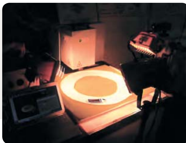
Thermal annealing of a perovskite film on a hotplate
