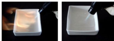
Fig. 1 \text{mol dm}^{-3} \text{ Li}[\text{TFSA}]/\text{EC-DMC} (left), and [\text{Li}(\text{G}4)_1][\text{TFSA}] (right).
