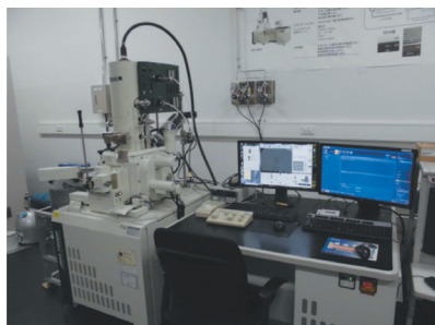
SEM (Scanning Electron Microscope) (National Institute for Materials Science) This SEM can detect elements over 50 eV and can detect Li, which is generally undetectable.
