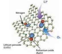
Schematic diagram of the surface of three-dimensional nanoporous graphene
