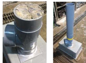
Water permeability test with a constant head
