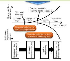
Mapped applicable monitoring technologies based on the progress of deterioration.
