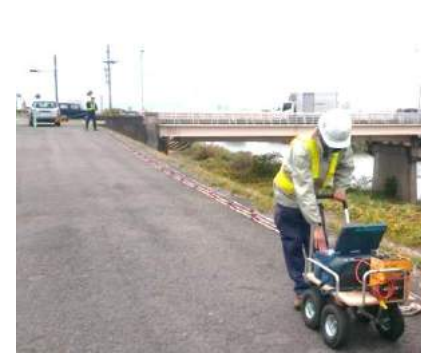
Land streamer type surface wave survey
