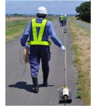
Trailing type electric survey
