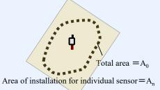
Suitable sensor intervals for multipoint measurement reduces the coverage of each sensor, thus improving system accuracy:
