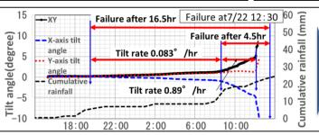
Early warning can be issued based on the relationship between tilt rate and remaining time to failure.
