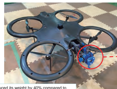
Reduced its weight by 40% compared to the previous flying robot
