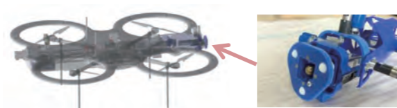
Flying robot under development Hammering test equipment
