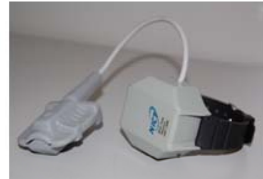
Wrist watch unit (SpO2, pulse, temperature)
