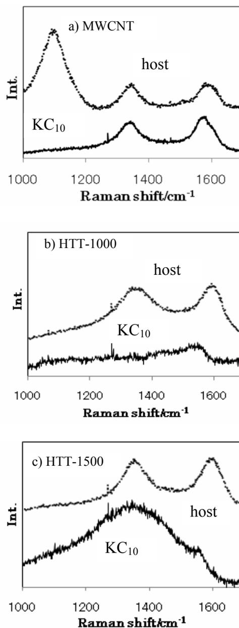
Fig. 1 Raman spectra of carbons and derived KC<sub>10</sub> samples.
