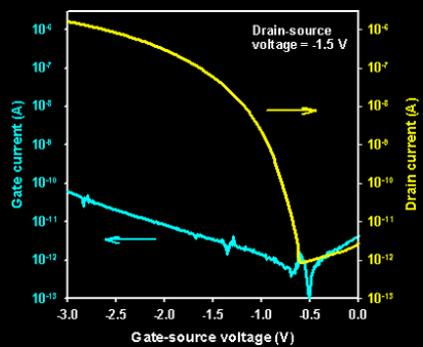
on/off current ratio =  $10^6$ ;  $I_D/I_G > 10^4$
