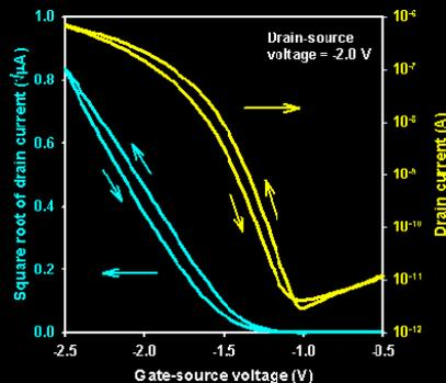
Subthreshold slope = 110 mV/dec
