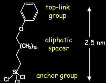
Molecular self-assembled monolayers with benzene "top-link" are perfectly **amorphous** (without grain boundaries) and free of defects over large areas (many square microns).
