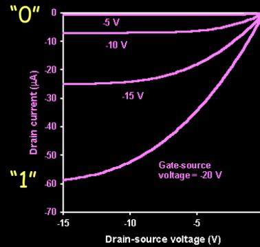
OTFT - electronic switch modulated by gate voltage
