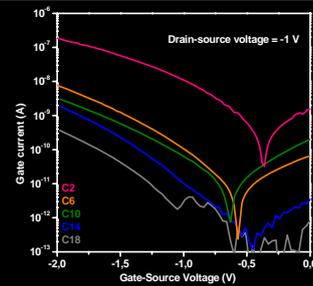
TFT gate leakage related to sub-nm changing in SAM dielectric thickness (40 x 100 μm area)
