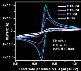
CV-characteristics independent method (electrode area ~ 5 cm<sup>2</sup>)
