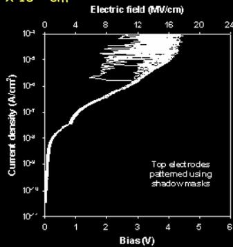
Current density as a function of voltage for 20 capacitors
