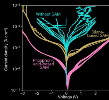
Density of packaging is **2.5 times larger** for phosphonic acid based SAM compared to silane based SAM (calculated from XPS data)
