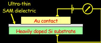
A current density of  $(8 \pm 1) \times 10^{-8} \text{ A/cm}^2$  was measured at 1V (corresponding to an electric field of 4 MV/cm). Dielectric breakdown occurs at  $14 \pm 2 \text{ MV/cm}$ .
