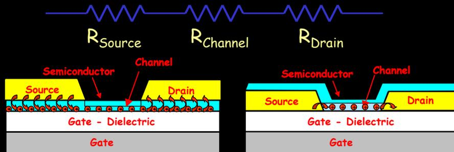
Charge injection (contact resistance) dominates the TFT performance!
