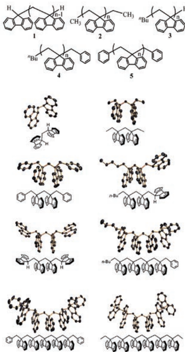
Fig. 2. Crystal structures of DBF oligomers having various terminal groups.
