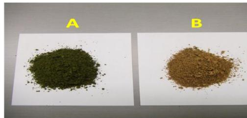
Residues after the SCF (CO<sub>2</sub>) extraction (A) and chloroform/methanol ( 2:1, v/v) extraction (B)
