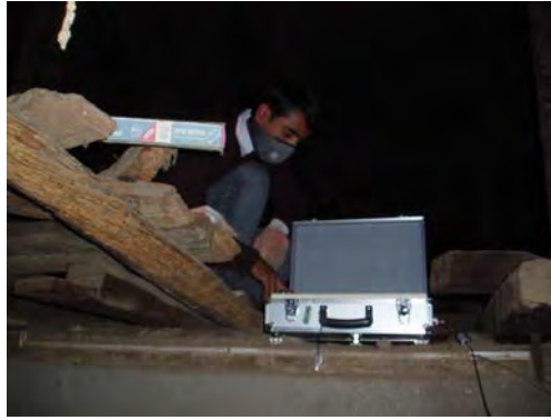
Microtremor observations in Jhatpole
