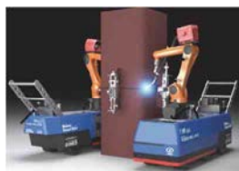
©Shimz Smart Site
