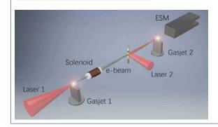
The experiment was carried out with the P-cube 80-TW Ti:Sapphire laser system at Osaka University, which can deliver 2 synchronized CPA laser beams from the same oscillator. The laser beam 1 was focused a He gas jet producing injector electrons. A solenoid collected and focus the electrons with desired energy to the booster plasma wake-field at 1 meter away. An electron spectrometer was installed just after the second gas jet.
