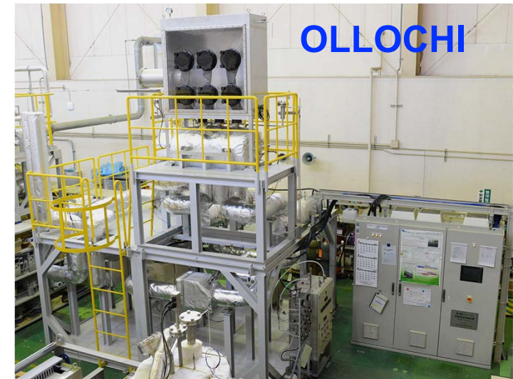
Oxygen-controlled LBE Loop for Corrosion tests in High temperature
