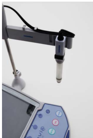
Ionic Liquid Salt Bridge for pH Detection
