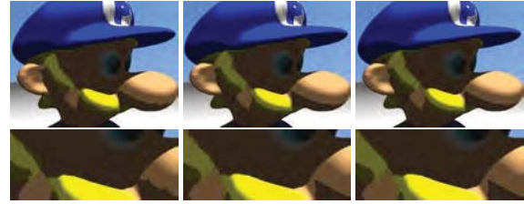
Figure 8: Using the discrete mesh silhouettes (left) causes self-shadowing artifacts on the Paolo model. The self-shadows can be improved using accurate silhouettes (middle), and further improved with smooth silhouettes (right).
