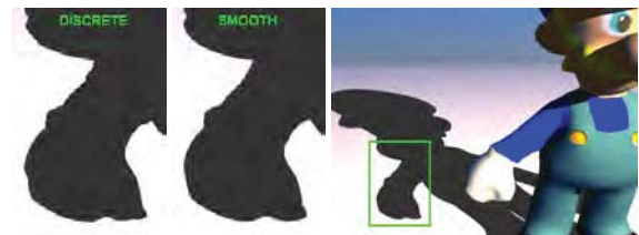
Figure 9: Closeup of a shadow of an arm of the Paolo model (6K triangles). While the discrete shadow is quite well tessellated (left), our algorithm improves the smoothness as can be seen in the closeup (middle) and the full image (right).
