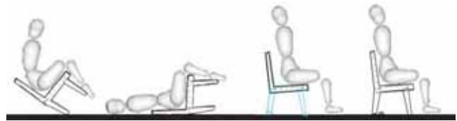
Figure 8. Testing and correcting an unbalanced chair.
