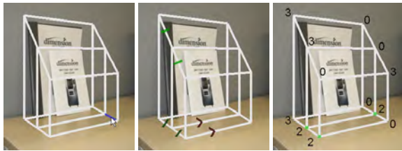
Figure 5: Left: Selecting edges with the mouse cursor. Middle: Three groups (each with different color) of two annotated lines. Green dash symbols are for same length lines and red arrows are for parallel lines. Right: Green highlighted vertices are ground vertices. Each vertex is labeled with the number of dimensions used in the full optimization. The total number of dimensions is reduced from 36 to 18.
