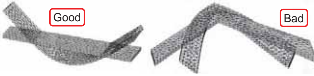
Figure 4: Perpendicular vibration mode is desirable (left), whereas in plane vibration mode is undesirable (right)
