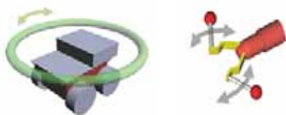
Figure 3: Virtual handles. Ring type for rotation of the vehicle, and lever type for manipulating end-effector of a robotic arm.
