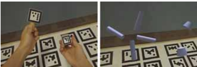
Figure 3. The user can translate and rotate the physical shapes in 3D space (left) and stamp virtual shapes (right) when desired.
