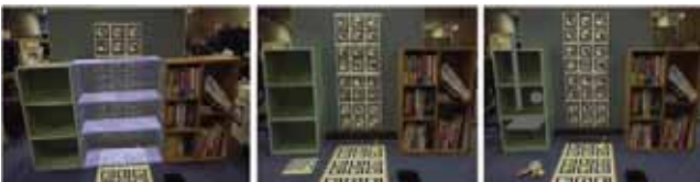
Figure 9. Image shown to users (left). Setup of Shape-stamping (middle) and Daichi-tools (right). For Daichi-tools, we needed a physical tool to represent the moving tool, and we used a cylinder primitive. Our implementation allows for moving a set of existing virtual shapes. For this study, we only used the virtual rectangular-board shape.
