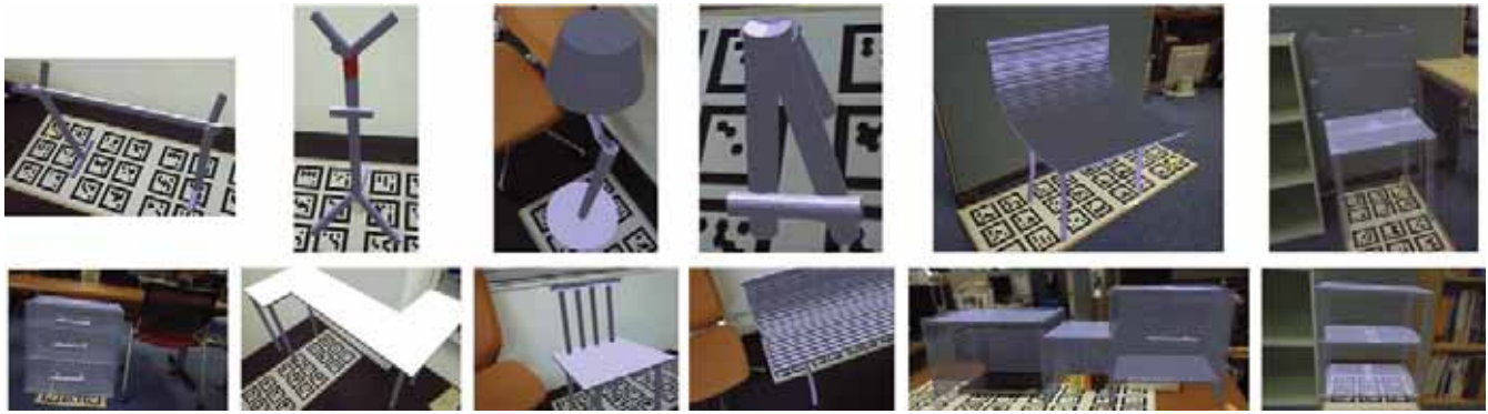
Figure 8. Do-it-yourself furniture and household products created by our system. From top left: clothes hangers, lamp, photo frame, chairs, cabinet, table, chair, bench, and shelves. Please see the video for some of the modeling processes.
